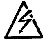
**WARNING:** A damaged power cord can lead to a hazardous electric shock. Check the power cord regularly. Do not operate the unit when the power cord is damaged. Always have a damaged cord replaced through a specialist. Do not wrap the cord around the unit and protect it from oil, heat and sharp edges. Do not carry the unit by the cord and do not use the cord to pull the plug from the outlet.
